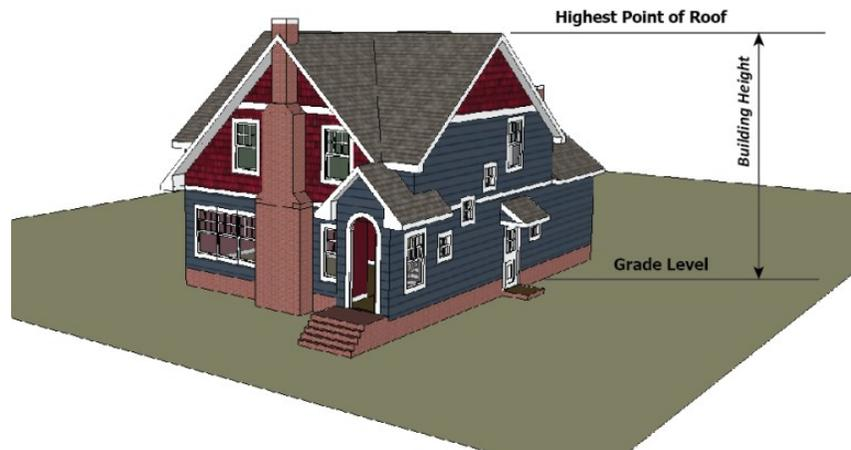
*Figure 5.05-J: Measurement of building or structure height*
