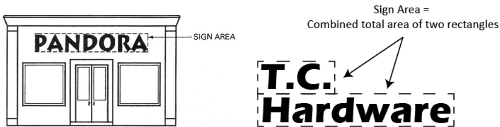
Figure 13.05-E: Illustration of sign area calculation for two differently shaped wall signs with individual letters.
