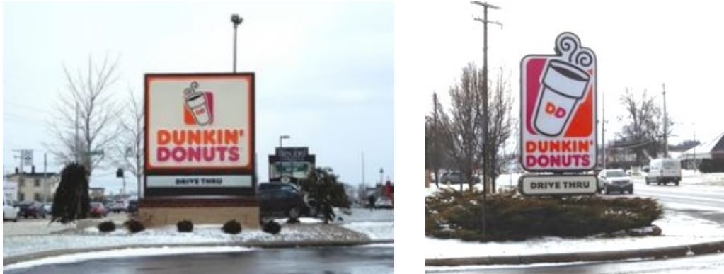
Figure 13.09-B: The sign on the left is a freestanding monument sign on a solid base. The sign on the right is a cabinet sign mounted on a pole, screened by landscaping. Both types are permitted.
