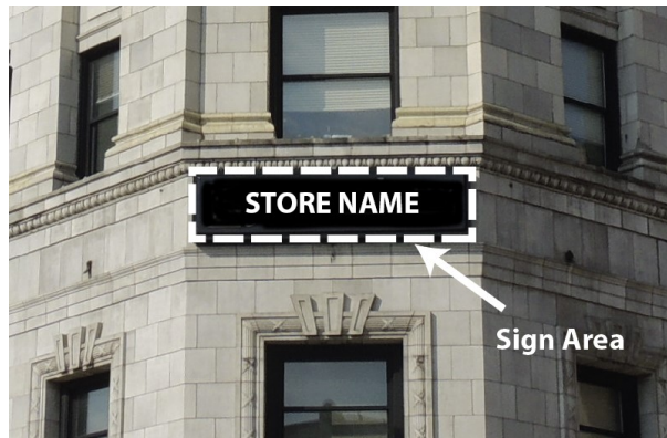
Figure 13.05-C: Illustration of computing the sign area for wall signs with a background panel or cabinet.
