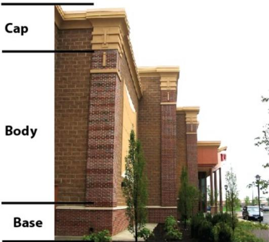
Figure 10-E: Image of a building with a clear, base, body, and cap
